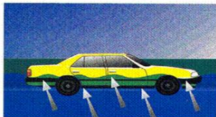
But the biggest factor is buoyancy. For each foot the water rises up the side of the car, the car displaces 1,500 lbs. of water. In effect, the car weighs 1,500 lbs. less for each foot the water rises.
