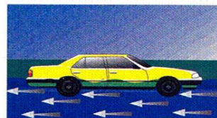
When a vehicle stalls in the water, the water's momentum is transferred to the car. For each foot the water rises, 500 lbs. of lateral force are applied to the car.
